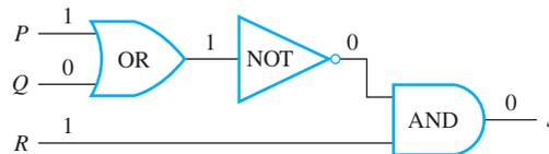
To construct the entire input/output table for a circuit, trace through the circuit to find the corresponding output signals for each possible combination of input signals.
