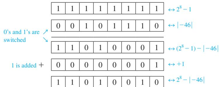
Because 127 is the largest integer represented in the 8-bit two's complement system and because  $127_{10} = 01111111_2$ , all the 8-bit two's complements for nonnegative integers have a leading bit of 0. Moreover, because the bits are switched, the leading bit for all the negative integers is 1. Table 2.5.2 illustrates the 8-bit two's complement representations for the integers from  $-128$  through 127.
