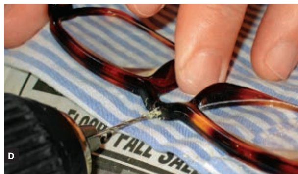
using the clamp and some rubber bands. Fig. C: Use enough glue so the joint is full, but be neat and don't get glue all over the place. Fig. D: Drill holes on either side of the repair for sewing the tension wrap.
