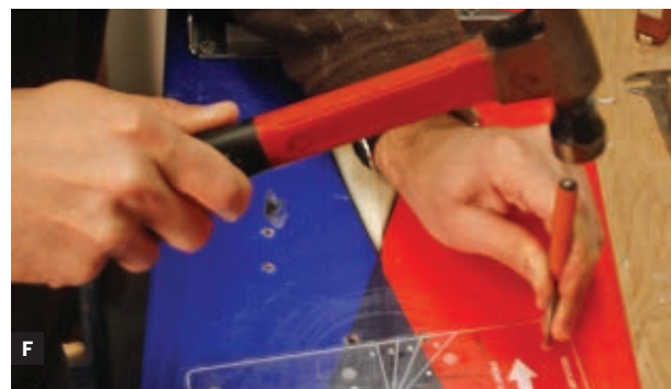
pivoting board hooks and other hardware. Fig. E: Mark holes for the touring brackets and climbing blocks using the paper template. Fig. F: Use regular or goofy stickers to mount binding pucks at the correct angle.
