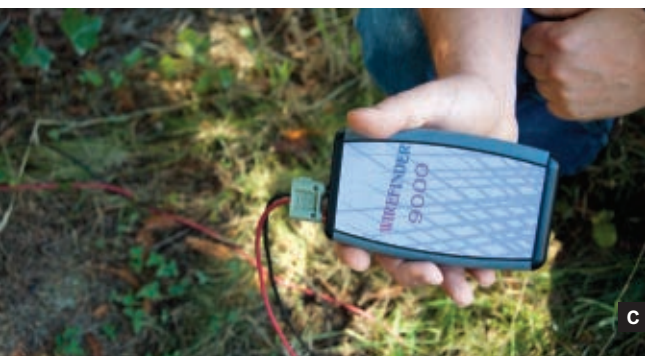
Fig. A: The completed WireFinder transmitter in a slick project enclosure. Fig. B: The completed transmitter, opened up to show component placement. Fig. C: Connect the buried wire or cable directly to the
