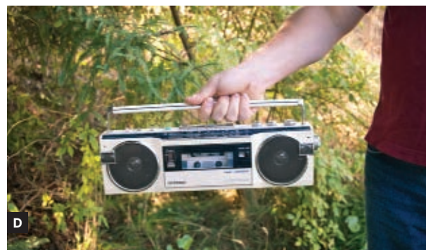
red terminal on the WireFinder transmitter. Fig. D: Follow the buried wire by listening to the tone that it's transmitting to your AM radio. If the tone drops off suddenly, start digging.
