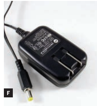
battery and wires for the charger (upper right), microphone (lower left), and speaker (lower right). Fig. E: The charging jack and flat washer spacer installed. Fig. F: The modified charger with coaxial power plug.
