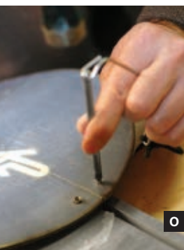
Fig. M: The toe of the binding should face the pin. To switch from touring to downhill mode, simply unlock the pin and slide it from the bracket. Fig. N: Pin locked in touring mode. Fig. O: Set the rivets for the tip clips.
