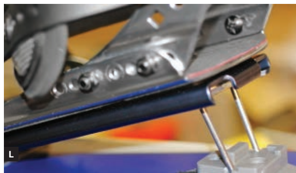
of the binding plate. Fig. J: Snowboard mode, bindings mounted to pucks. Fig. K: Touring mode, bindings mounted to touring brackets. Fig. L: The climbing bar is very useful for the steeper uphill sections while touring.
