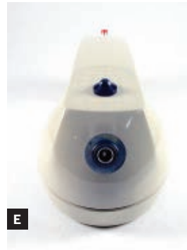
battery and wires for the charger (upper right), microphone (lower left), and speaker (lower right). Fig. E: The charging jack and flat washer spacer installed. Fig. F: The modified charger with coaxial power plug.
