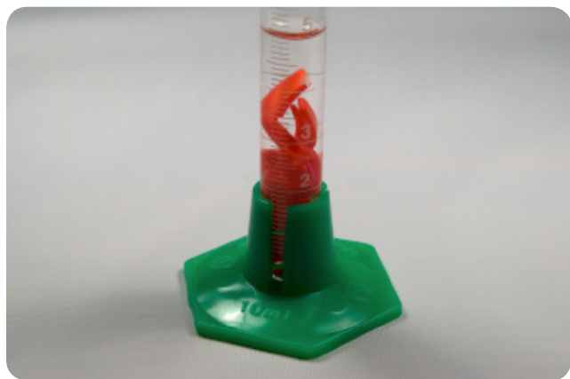
Figure III-1-1: Determining the amount of liquid displaced by a small specimen
