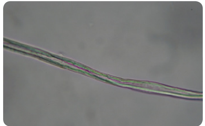
Figure II-7-11: At focus, the Becke line appears near the edge of the fiber
