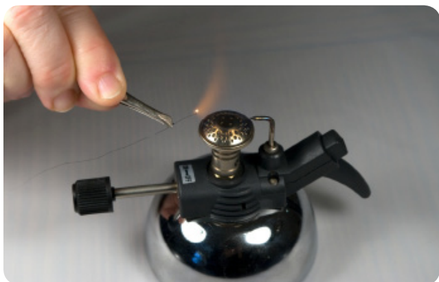
Figure II-6-1: Barbara test burning a fiber specimen
