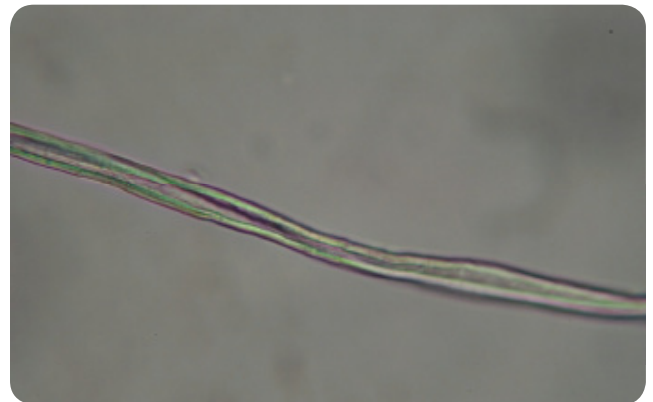
Figure II-7-12: As focus is opened, the Becke line moves toward the center of the fiber
