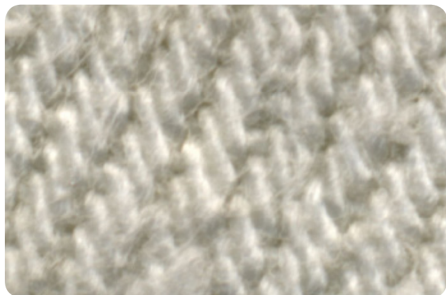
Figure II-6-3: The same fabric specimen after dye stripping
