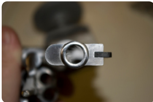
Figure VI-0-1: Looking down the muzzle of a .44 revolver at the spiral rifling lands and grooves
