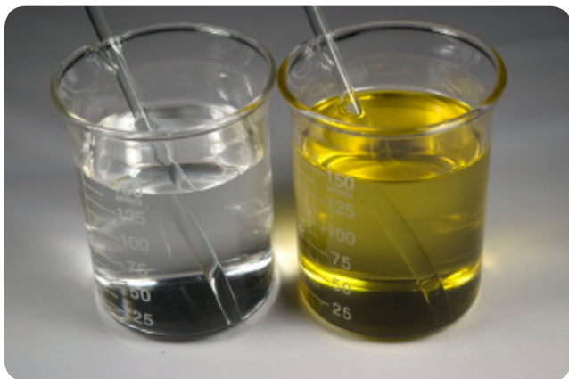
Figure II-7-8: Glass rods in water (left) and olive oil
