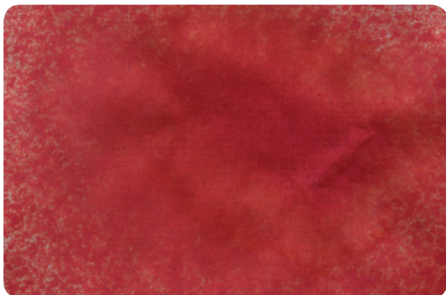
Figure IX-1-4: Orange stains indicate the presence of nitrites in a simulated GSR specimen (sodium nitrite on paper)
