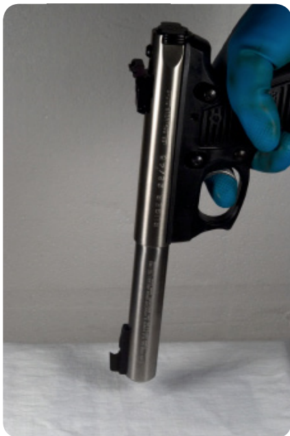
Figure IX-1-1: Firing a test shot with the muzzle in close contact with the cloth specimen
