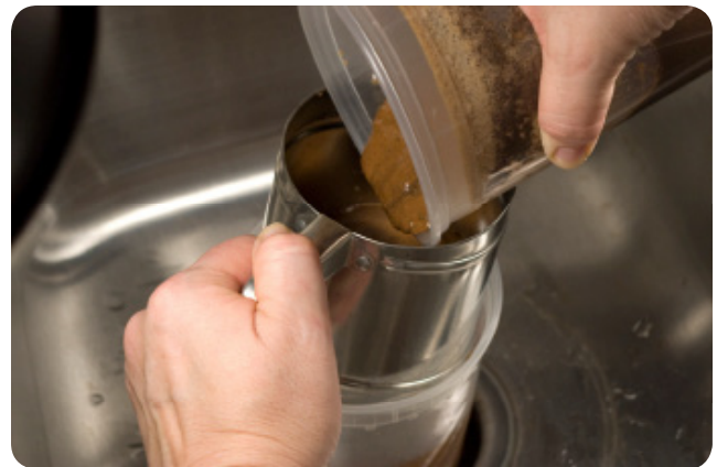
Figure I-2-3: Wet sieving a soil specimen
