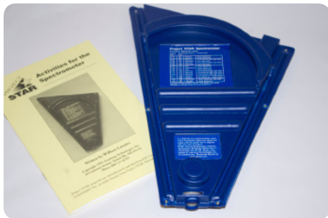
Figure 2-7: The Project Star Spectrometer, an inexpensive spectrophotometer
