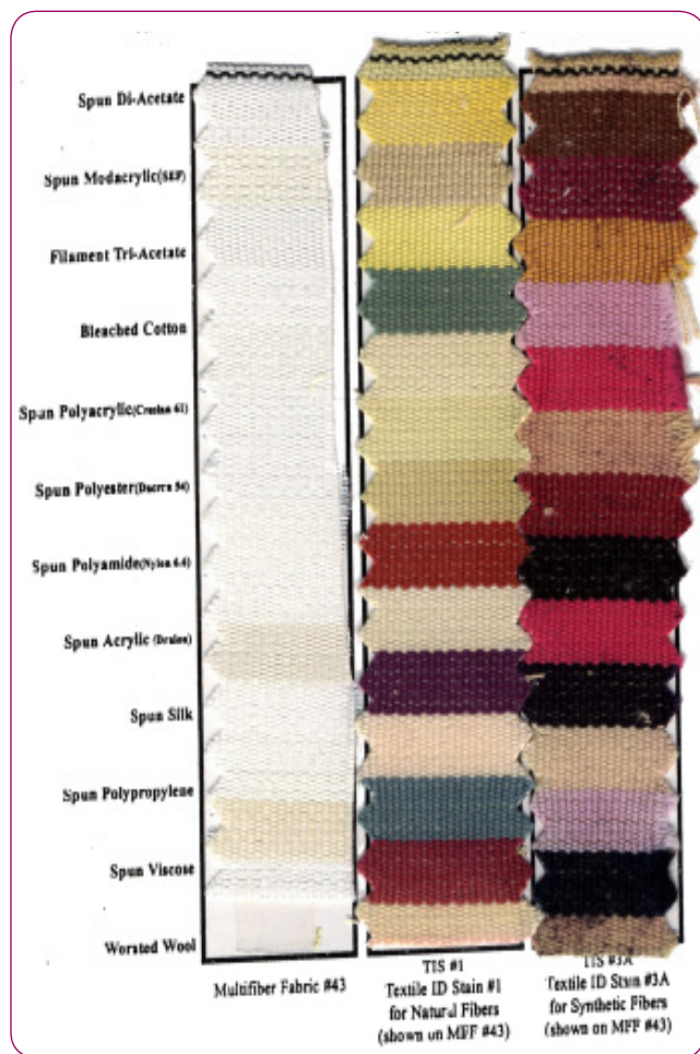
Figure II-6-4: Multifiber Fabric #43 specimens before dyeing (left), dyed with TIS #1 stain (center), and dyed with TIS #3A stain
