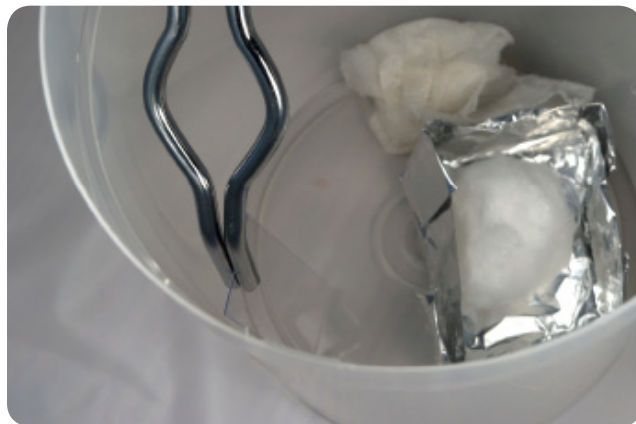
Figure IV-4-1: Placing the specimen in the superglue fuming chamber
