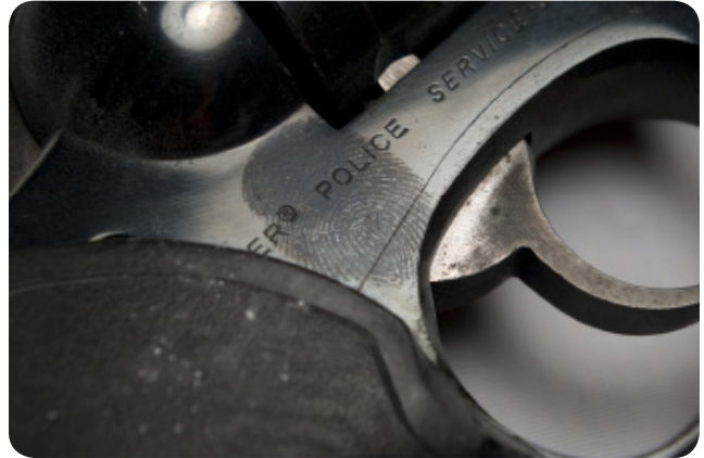
Figure IV-1-2: Dusting prints on the surface of the specimen
