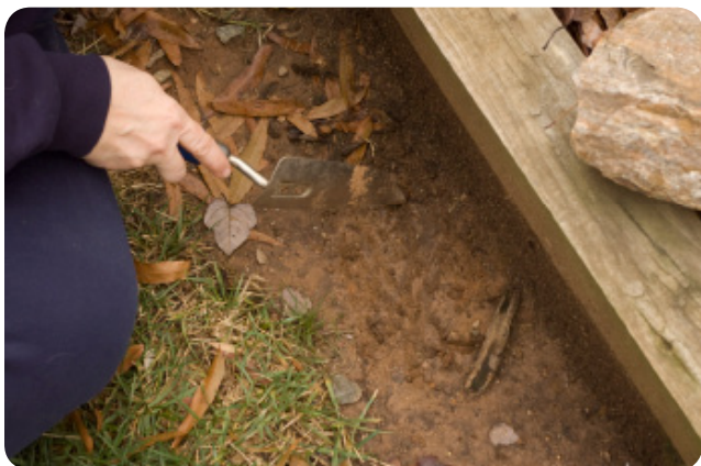
Figure I-1-1: Barbara removing extraneous material before gathering a soil specimen
