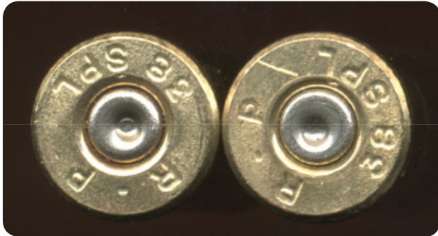
Figure VI-0-2: The firing pin impressions made by a revolver on the primers of two .38 Special cartridges
