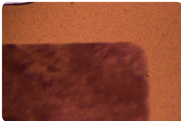
Figure VI-2-2: Color negative film at 40X showing no individualizable mask roughness
