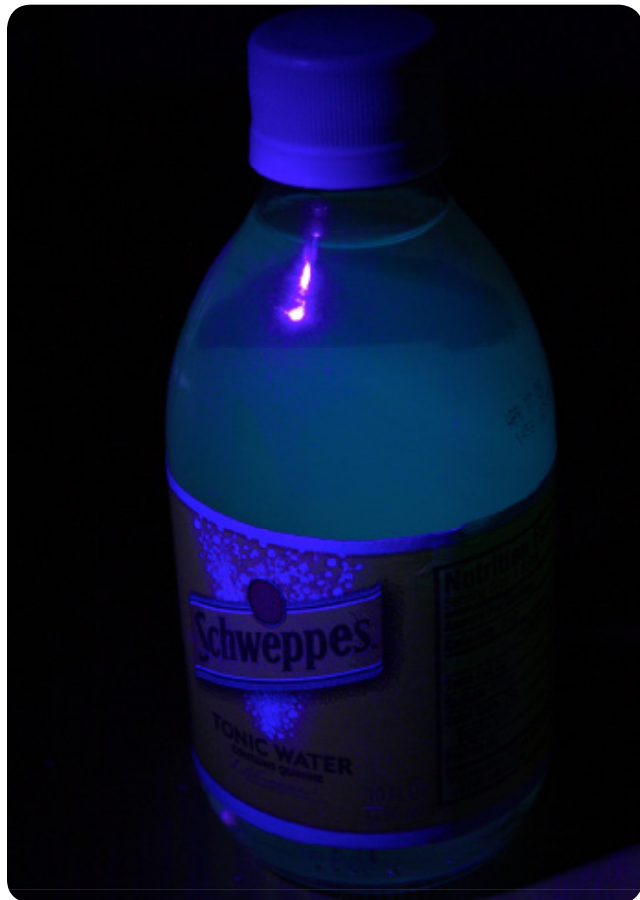
Figure VIII-2-2: Quinine in tonic water fluorescing under UV light
