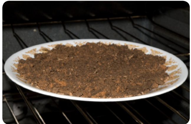
Figure I-1-3: Soil specimen drying in the oven
