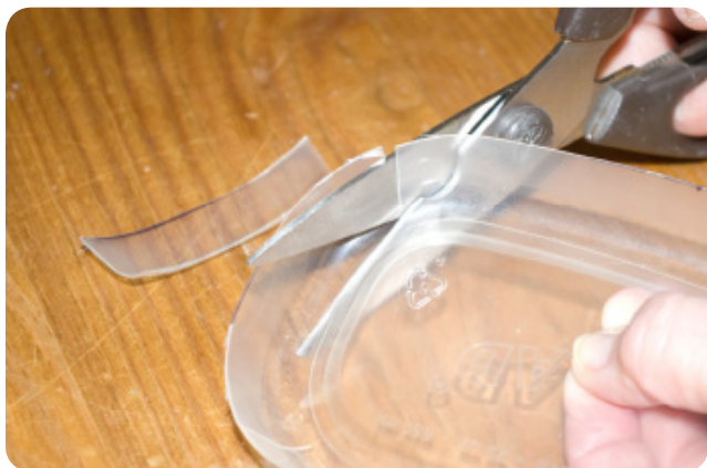
Figure XI-4-3: Removing the ends from the gel casting tray
