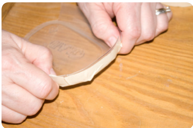
Figure XI-4-4: Taping the ends of the gel casting tray into place
