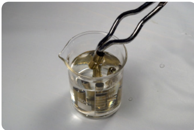
Figure IV-6-1: Treating cartridge cases with acidified hydrogen peroxide
