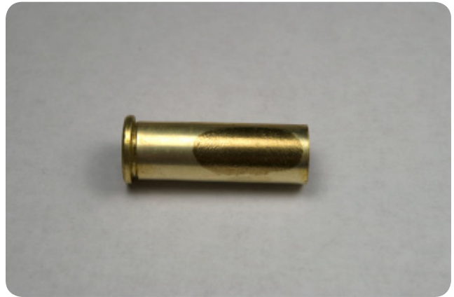
Figure IV-6-2: Partial latent fingerprint on a cartridge case revealed by acidified hydrogen peroxide development
