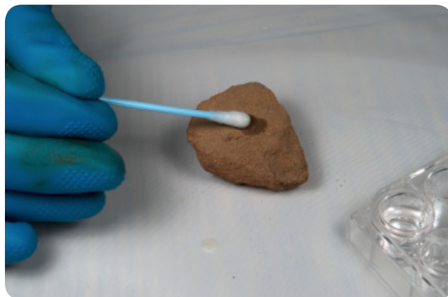
Figure IX-2-2: Obtaining explosives residue specimens with a cotton swab
