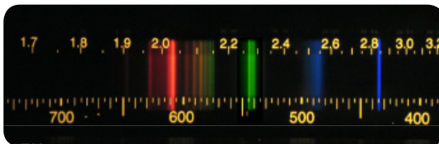
Figure 2-6: The spectrum of a compact fluorescent lamp, showing strong mercury lines (image courtesy Rob Brown)
