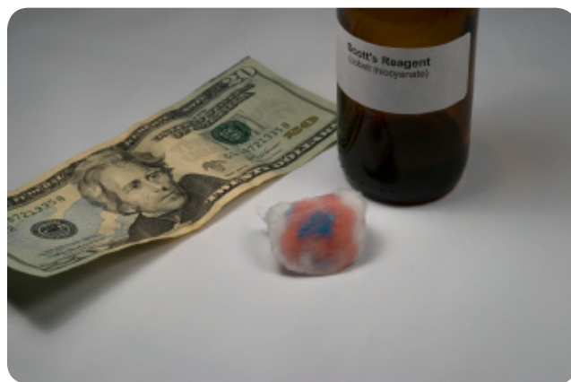
Figure VII-2-1: A cotton ball showing a positive test for diphenhydramine
