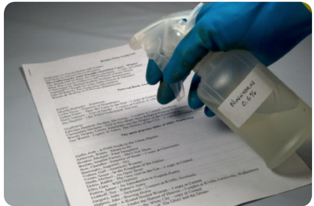
Figure IV-3-1: Spraying a specimen with ninhydrin solution
