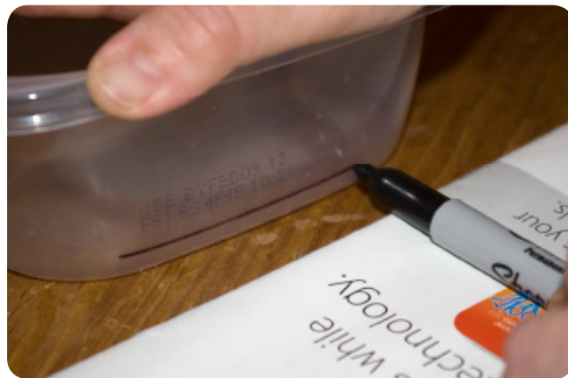
Figure XI-4-2: Marking the gel casting tray for depth
