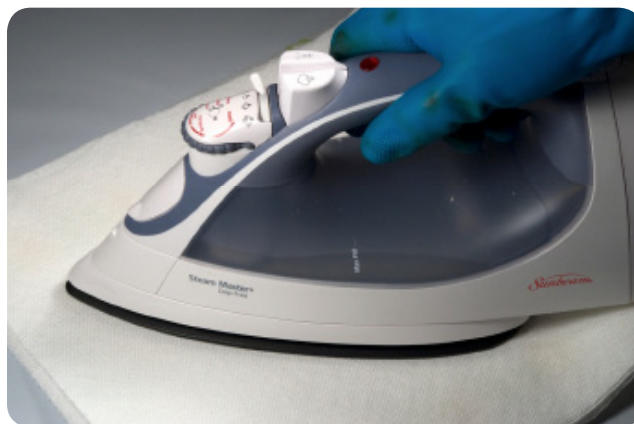
Figure IX-1-3: Pressing the Griess reagent test paper in contact with the cloth specimen
