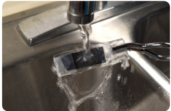
Figure IV-5-1: Rinsing a specimen after treating it with gentian violet solution
