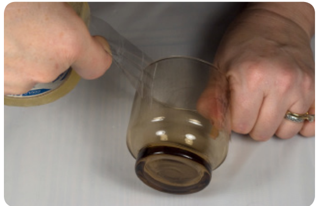
Figure IV-1-3: Barbara lifting a dusted fingerprint from a specimen
