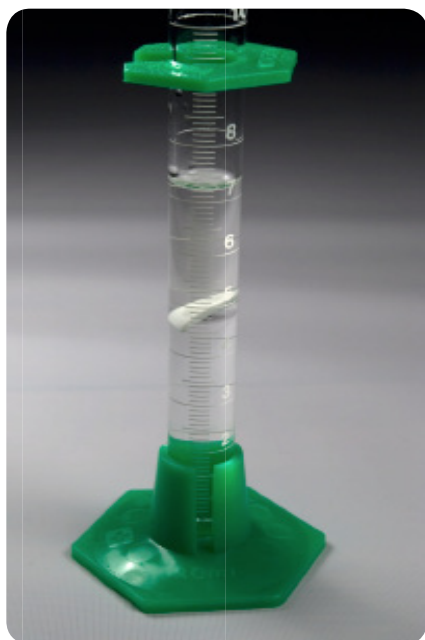
Figure III-1-2: When the density of the specimen and fluid are the same, the specimen neither rises nor sinks
