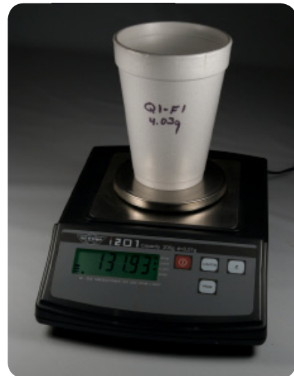
Figure I-2-4: Determining the mass of a soil specimen fraction
