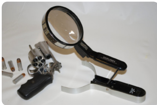
Figure 2-4: A stand magnifier allows you to work with both hands free
