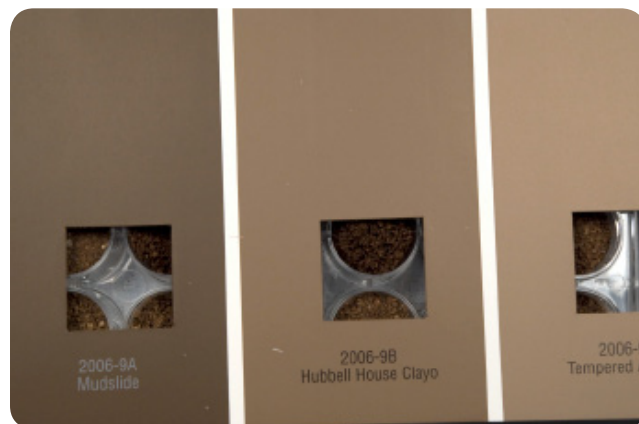
Figure I-2-2: Comparing paint chip samples against a soil specimen
