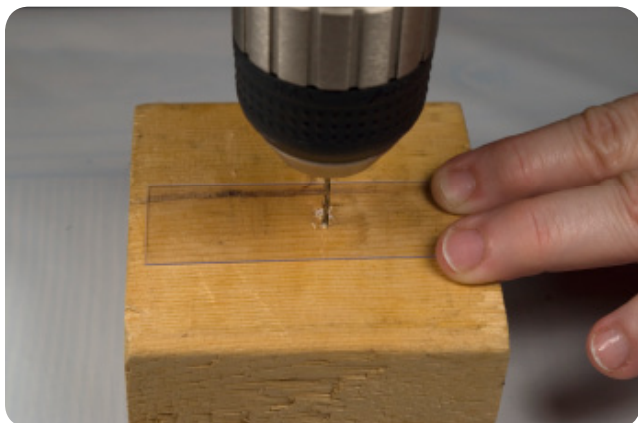
Figure II-7-6: Drilling a plastic microscope slide for use as a sectioning slide
