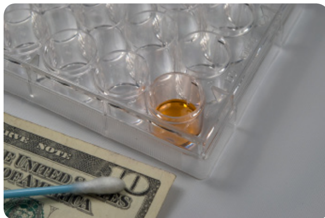
Figure VII-2-2: A positive Marquis reagent test for methamphetamine
