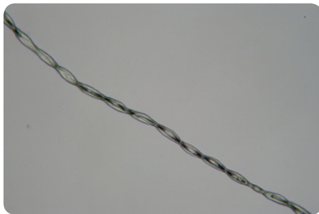
Figure II-7-3: A cotton fiber at 100X magnification
