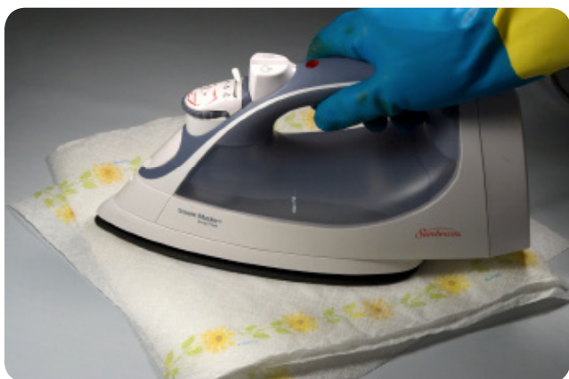
Figure IV-3-2: Applying moist heat to develop the fingerprints treated with ninhydrin solution
