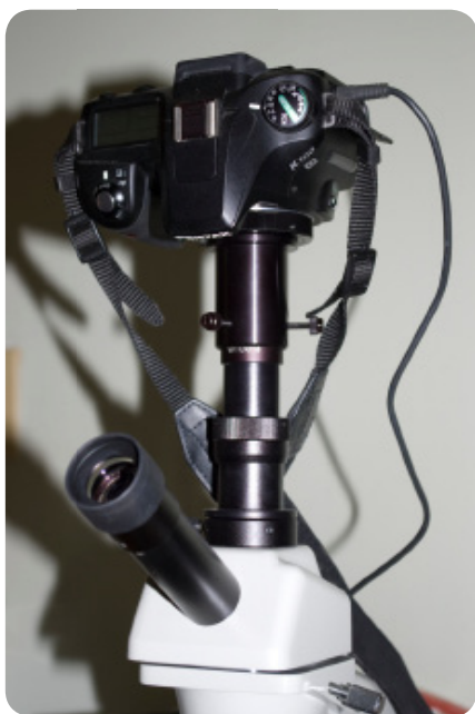
Figure 2-5: A DSLR coupled to a microscope with a T-ring and microscope adapter
