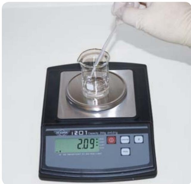
I wasn't so lucky with another pipette, which was rated to deliver 43 drops/mL but in fact delivered closer to 44 drops/mL, at least using my dropping technique. Still, once the actual delivery rate is known, the nominal delivery rate is immaterial. Because I've calibrated them, I can use those pipettes to deliver accurately known small amounts of liquid reliably.
