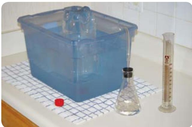
My first thought was to use an inverted 100 mL graduated cylinder as the gas collection vessel, which would have made it easy to measure directly the volume of gas produced. A few quick calculations convinced me to use a larger gas collection vessel. I reasoned as follows:
