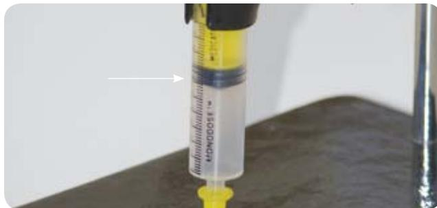
7. Clamp the syringe as shown in Figure 14-2. Make sure that the cap of the syringe is pressing directly against the base of the ring stand. Otherwise, when you add mass to the container, the cap might pop off the syringe.
