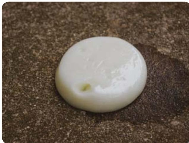
the beaker. If not, tap the beaker gently to release the gelled sol. When the gelled sol separates, note that it retains its form, as shown in Figure 18-5. There should be little or no liquid gasoline remaining. (The stain visible to the right of the gelled sol in Figure 18-5 is a small amount, probably less than 1 mL, of liquid gasoline that was not incorporated in the sol.)
