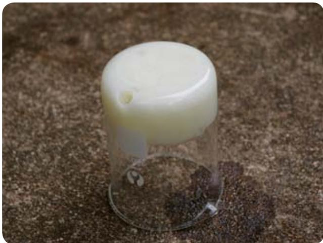
8. If you are not already outdoors, take the beaker to a safe outdoor location with a nonflammable surface such as dirt, gravel, or concrete. (Remember that asphalt, made from tar, is flammable.) Invert the beaker, and wait a few moments to see whether the gelled sol separates from
