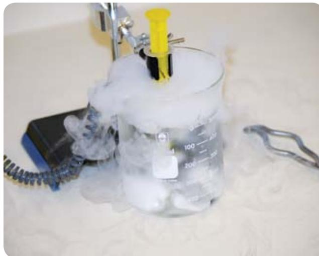
7. Remove the syringe from the dry ice bath and set it aside to return to room temperature. When it has done so, verify that the volume has returned to the original reading. (Press the plunger gently once or twice to ensure that it can move freely; the readings should be the same each time.)
