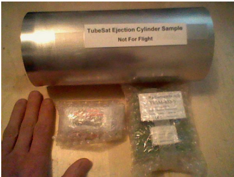
Figure 3-2. Close-up of primary components for a TubeSat platform (sans instrumentation)
