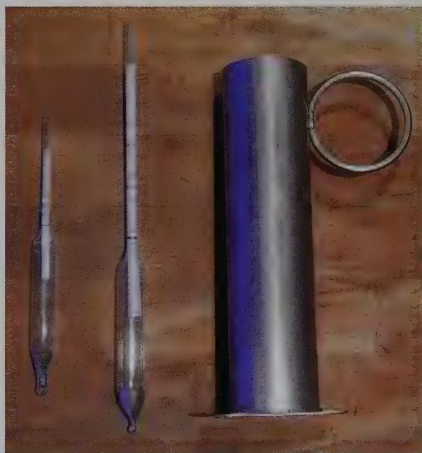
Figure 4.47. Hydrometers for measuring percent sap (left) and sugar content in finished syrup (middle). Purchasing the metal tube shown is helpful, as it makes it easy to place the hydrometer in and pour sap or syrup until full to get a reading.
