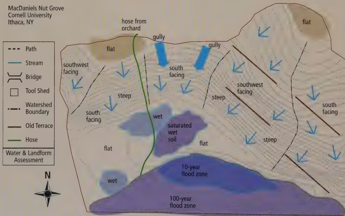
Figure 10.3. Water assessment map for the nut grove. Areas where water was pooling and causing erosion gullies are noted, along with level areas at the top of the slope (good for dropping materials) and the general lack of on-site water for irrigation. The site is overwhelmingly steep sloped with south and southwest aspects. The lower section near the creek is wet and prone to flooding.
