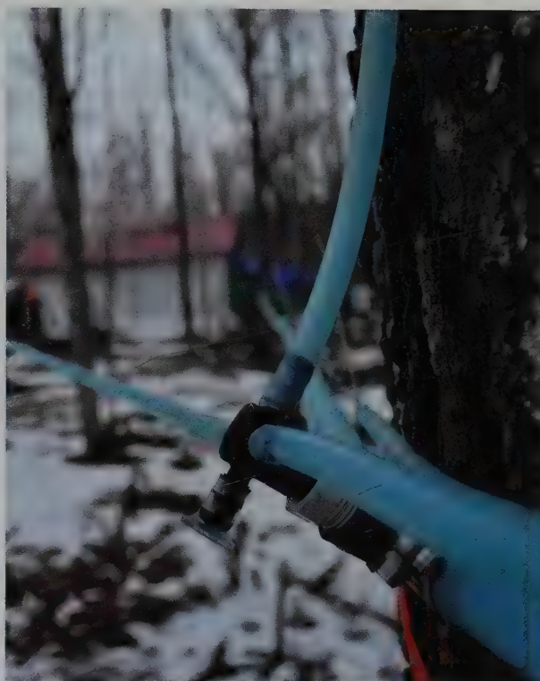
Figure 4.43. Maple-specific tubing strung between trees at Sapsquatch Pure Maple Syrup. Smaller \frac{3}{16} -inch-diameter tubing comes from the trees as “drop lines,” which feed the larger \frac{1}{2} -inch line running from left to right toward the sugar shack. Photograph courtesy of Jen Gabriel
