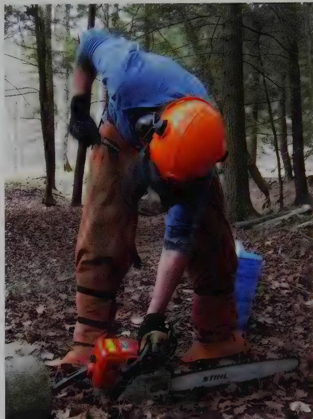
Figure 10.20. The safest way to start a saw is on the ground. Be sure that the chain brake is engaged and that the operator is wearing all the necessary safety gear. Photograph courtesy of Jake Delisle
