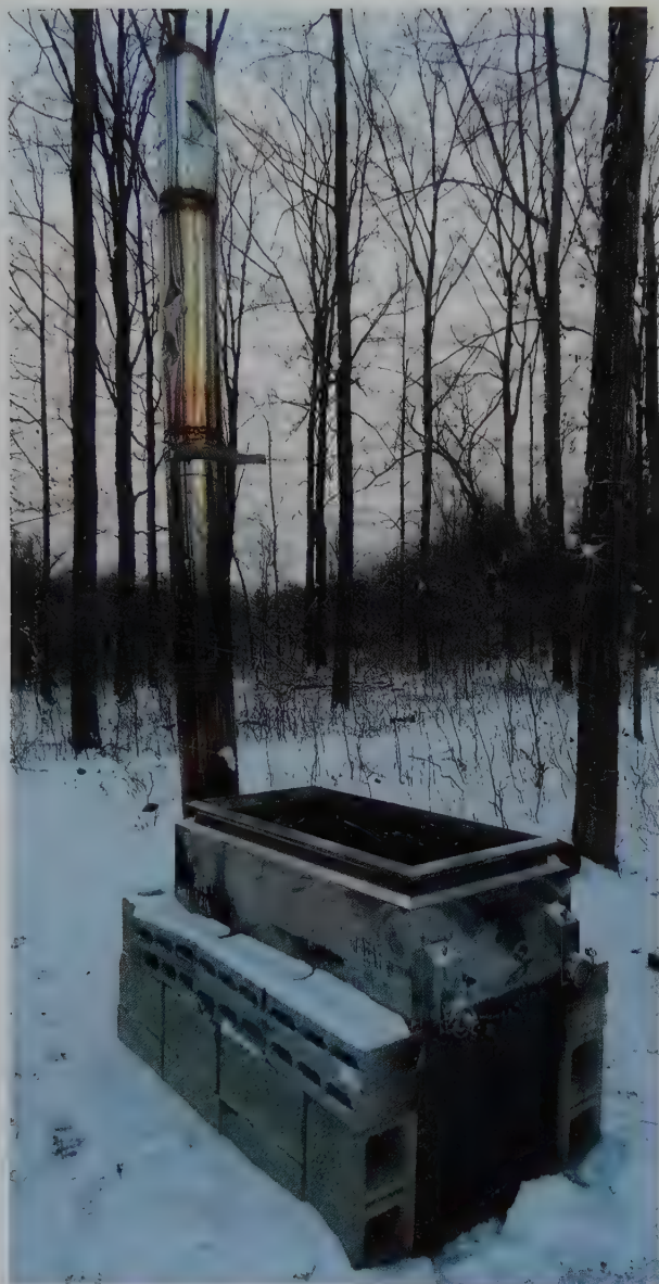
Figure 4.41. A medium-scale boiler setup at Wellspring Forest Farm, designed to handle the sap from about a hundred trees. The pan was bought used from a maple producer, the firebox is made of cinder blocks, and the chimney stack was reclaimed from neighbors when they replaced their chimney.
