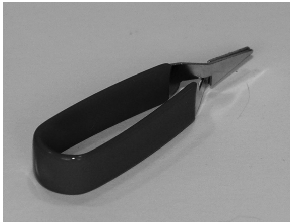
FIGURE 4.11 A heat sink with an insulated handle.
