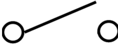
FIGURE 6.1 The symbol for an open switch in a circuit diagram.
