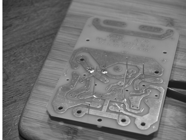
FIGURE 13.2 Bottom of the PCB. Note the leads and the copper traces and the first soldered joints in the upper left side of the PCB.
