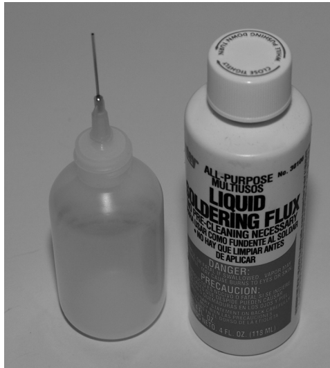
FIGURE 12.3 A flux bottle and liquid soldering flux.
