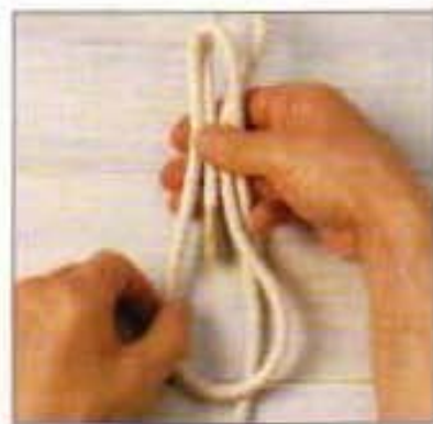
2 Make a loop of the required size with the long end of the rope.
