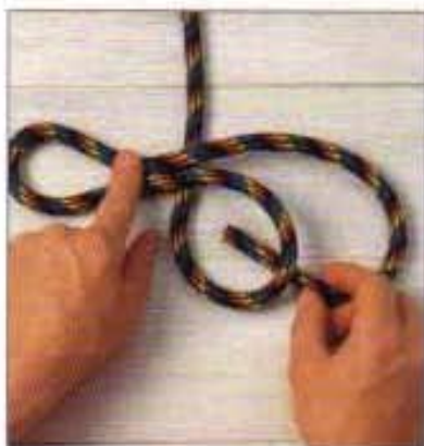
2 Reduce the size of the lower loop, secure the lefthand bight, and bring the working end around to create a second loop on the righthand side of the emerging knot.
