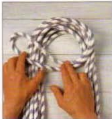
2 Bring the right back upon itself so as to create a loop.
