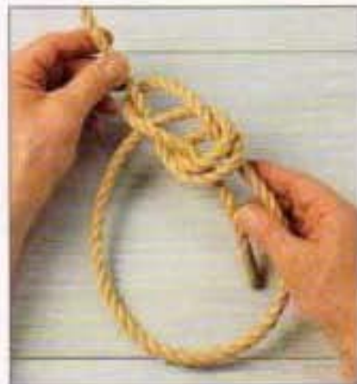
6 Then tuck it down through the double loop, beside its own other part, with a moderately long tail end.
