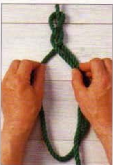
5 Repeat step 3, complying once more with the principle that the least used strand becomes the next working one.
