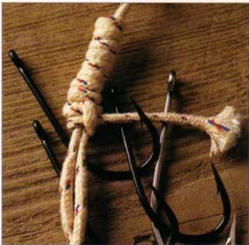
4 An overriding layer of wrapping turns should appear where the hands are focused. Hold the standing part taut and feed the working end at right angles into these turns under steady tension, keeping them tight and close together.
