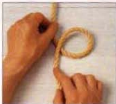
1 Form a small overhand loop with the working end of the rope.
