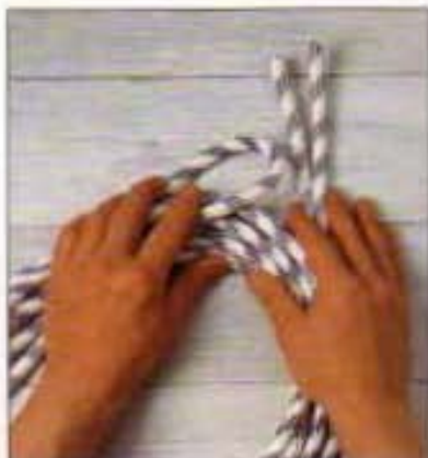
1 Middle the rope prior to coiling and then coil it doubled.
