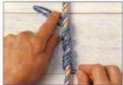
5 Complete four or five turns with the sling around the rope.
