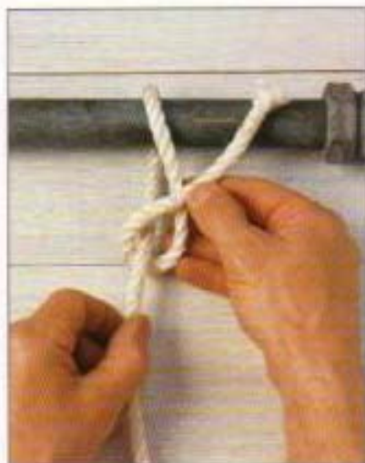
2 Take the end around its own standing part and make a small loop.
