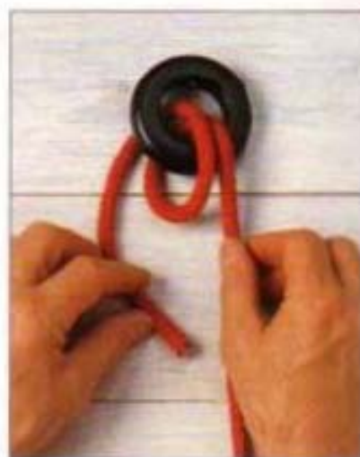
2 Lead the end through the ring a second time to create a round turn.
