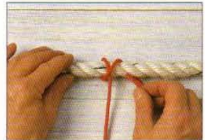
4 Pass the working end down behind the foundation to emerge at the front and to the right of the standing part.
