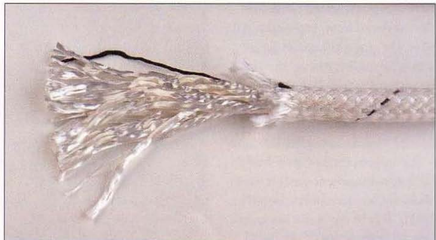
A 14 mm ( \frac{1}{2} in) diameter, soft matt polyester, 16-plait sheath encloses a hawser-laid core of several thousand high-tenacity polyester filaments.
