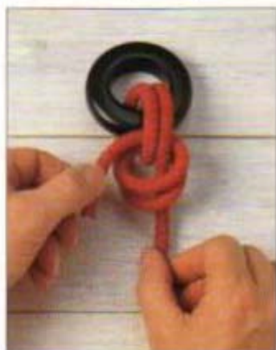
4 Then tuck the end a second time to create what is in effect one round turn through another round turn.
