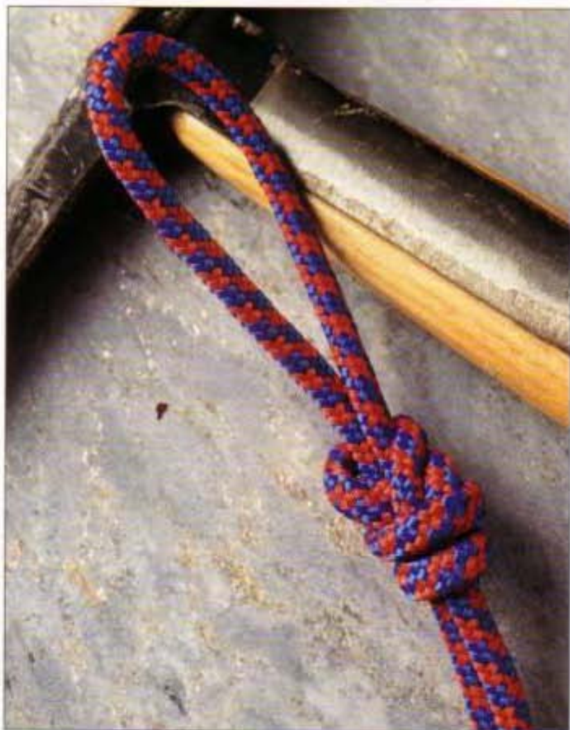
1 Make a generous bight in the end of the cord or rope.
