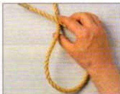
1 Bring the working end across the standing part of the rope to form an overhand loop.
