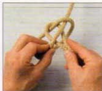
6 Draw the marlinespike hitch down over the bight. Note the untypical face of this bowline, when tightened, with its distinctive trefoil crown.
