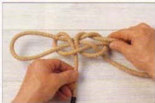
7 Take the working end down through its own loop to tie a half hitch.
