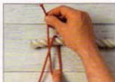
3 Pull a fairly long bight down from the lower part of the turn just made.
