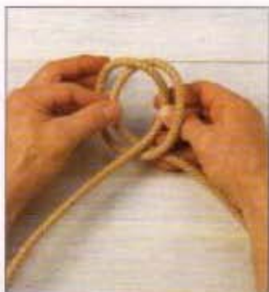
3 Partly overlap the two loops, the lefthand one in front of the righthand one, and prepare to pull the leading edge of the lefthand loop (from the front to the back) through the righthand loop, at the same time pulling the leading edge of the righthand loop (from the back to the front) through the lefthand loop.
