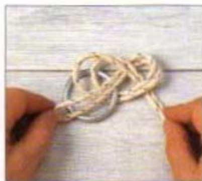
3 Then tuck the bight through the loop to tie an overhand knot around the ring.
