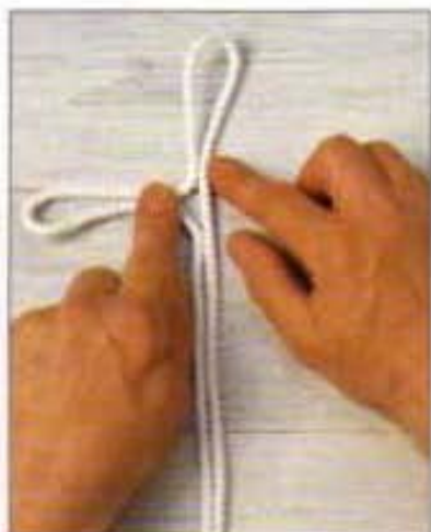
2 Pull out and retain a second bight in the lefthand leg of the cord.
