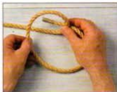
2 Rotate the hand clockwise and so produce a smaller loop in the standing part of the rope.
