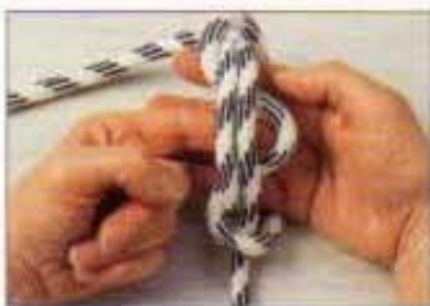
6 Tuck the lefthand rope part through (from left to right) beneath the other two turns.
