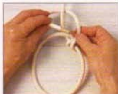
5 Complete two turns around the standing part of the rope, and divert the working end to pass around behind the standing part.
