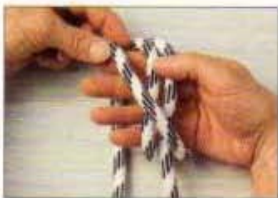
5 Carry this over to become the lefthand rope part.
