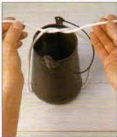
1 Place the lifting line beneath the load and tie a half knot on top.
