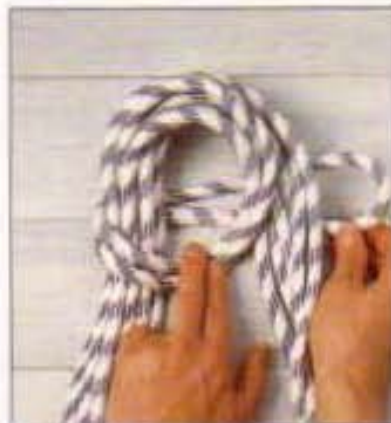
3 Lead the working right around the back of the coil to the other side.
