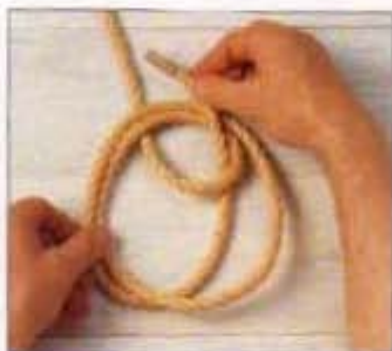
4 Bring it up and through the cinch as if tying a common bowline.
