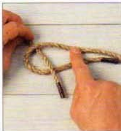
2 Tuck the working end up through the bight, angling it towards the other short end.
