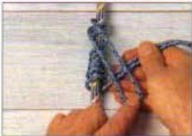
6 Tighten and neaten the wrapping turns (not perfectly illustrated) and bring the working bight down to the standing part of the sling.
