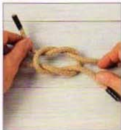
4 Finally, tuck the working end back through the bight to emerge alongside its own standing part.
