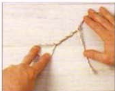
3 Spread the loop. In practice, this must be done with the feet, while both hands are free to control the two upper ends of the line. Start to enlarge the loop to unwind the initial twists.
