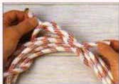
4 Where the two ends meet opposite the original reef (square) knot, tie another half-knot.
