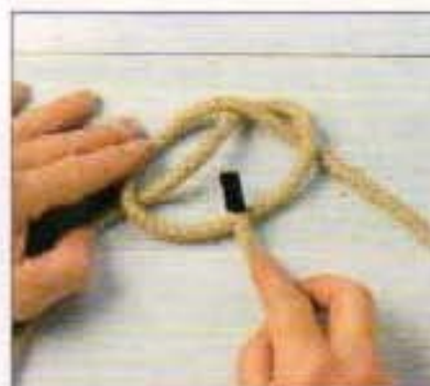
3 Lift the standing part of the rope up slightly within the loop.
