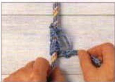
7 Tuck the remainder of the sling through the working bight to complete this friction hitch.
