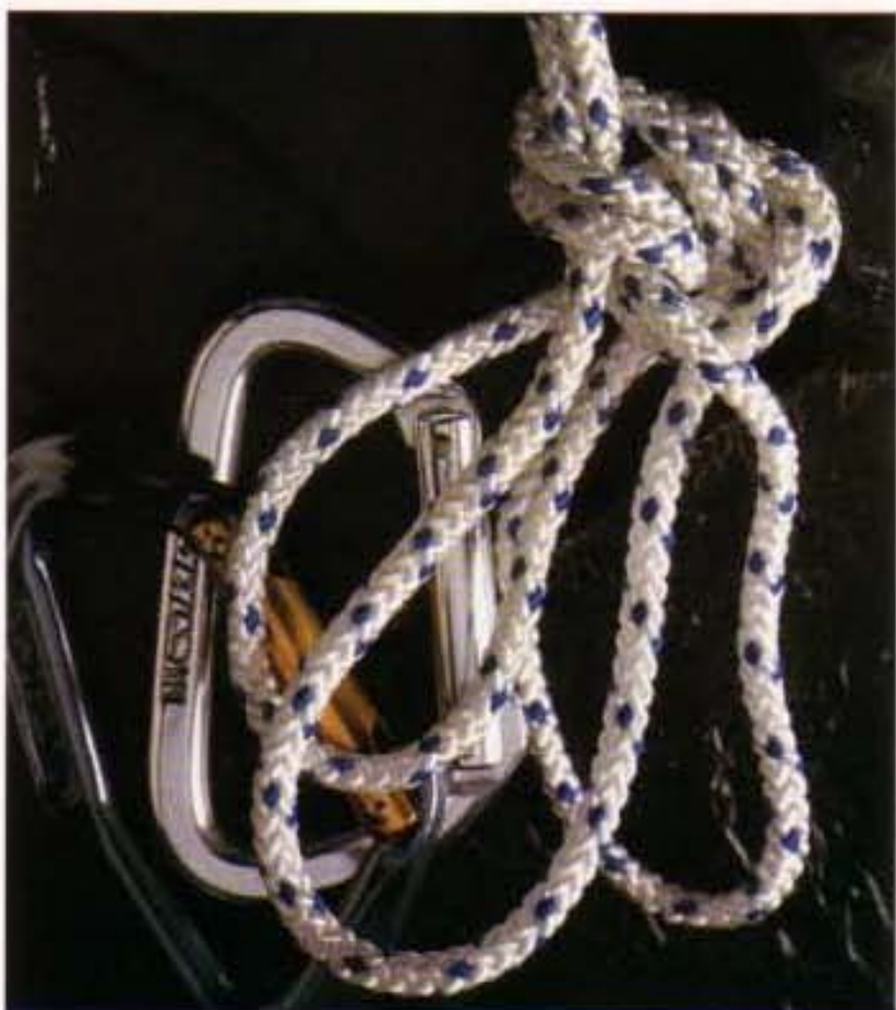
4 Pull up the bight, tipping the standing parts into the bowline form.
