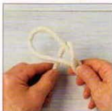
2 Begin to wrap the twin legs of the loop with the working end.
