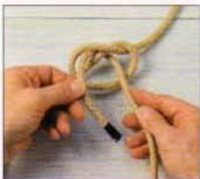
5 Let the working end be pulled into a bight by the marlinespike hitch.
