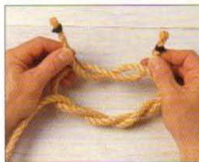
4 Tie a final half knot, of opposite handedness to the first couple, with the two parts twining righthanded (clockwise). To tighten the knot, first hold each working end with its adjacent standing part; but finally just pull on the standing parts, allowing the upper half knot to twist slightly so that it overlays the completed knot diagonally from corner to corner.
