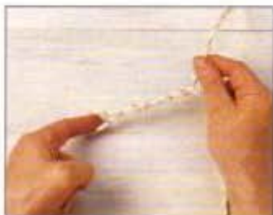
1 Make a bight over 50 cm/20 in long. Insert a finger in the end of the bight and begin to twist a loop around.
