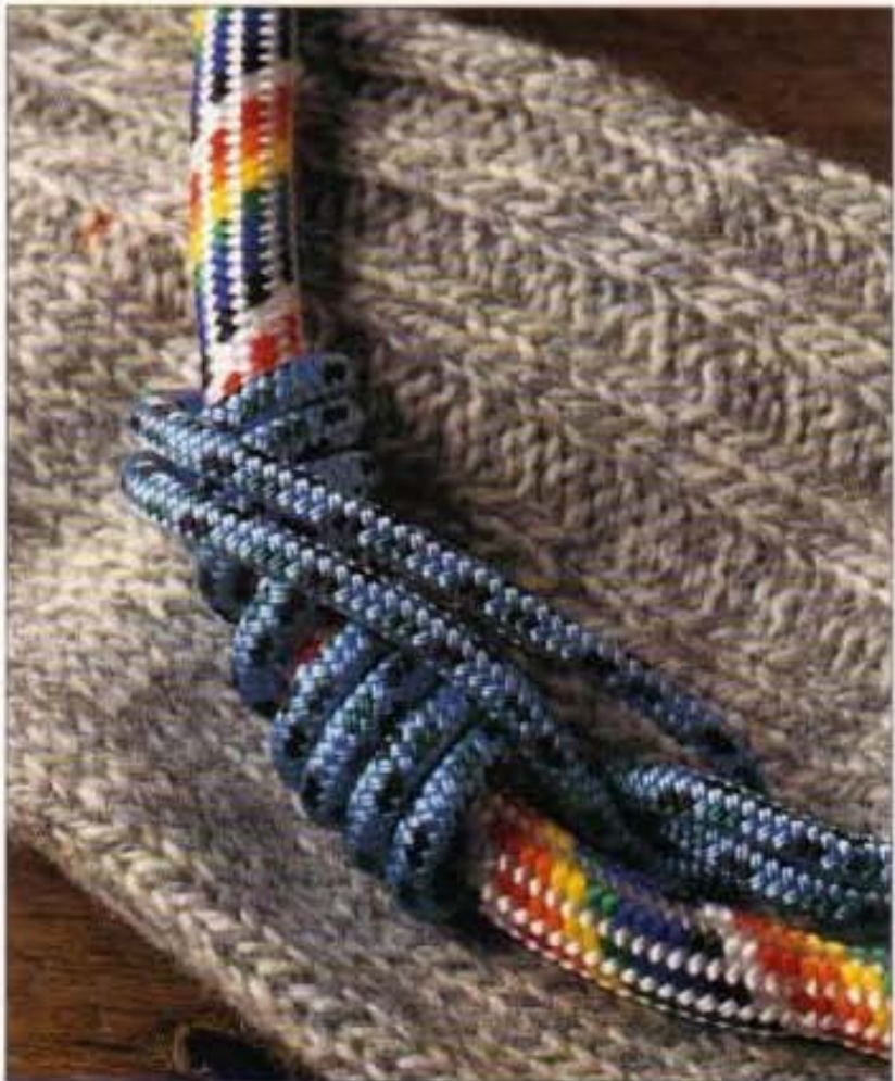
4 Ensure that both legs of the sling remain flat and parallel, with no crossovers, as the wrapping proceeds.
