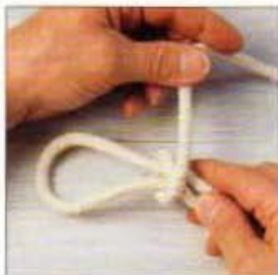
3 Take care to trap the third cordage part in the groove between the other two parts.
