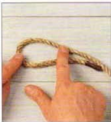
1 Make a small bight in one end of the cord or line.
