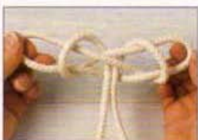
8 Pull the two loops outwards until they are the required size; pull down on the standing parts to tighten the knot. If one end is close to the knot, secure it to the adjacent standing part with a double overhand knot.
